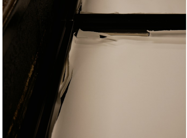
Metal rods used for securing the sample material
